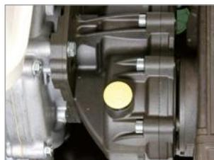
EQUIPADO CON UN REDUCTOR PARA PROLONGAR LA VIDA ÚTIL DE LA BOMBA
